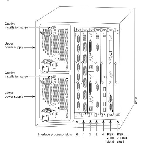
Figure 1 Cisco 7000 with RSP7000 and RSP7000Cl Installed
